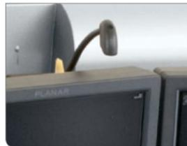
The Adaptive Lighting System adjusts ambient light to match the density of the on-screen image.
